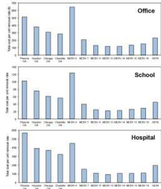
Figure 20. Total annual cost per unit removal rate (5 per 1/hr) of outdoor air ventilation and HVAC filtration products in each of the three hypothetical case study environments
