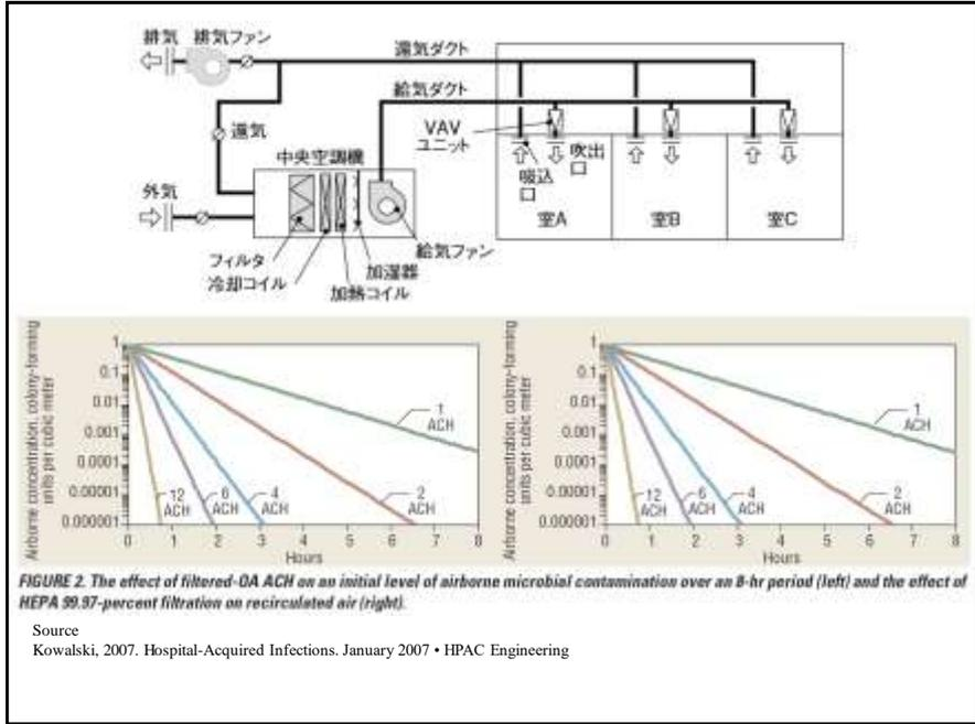
FIGURE 2. The effect of filtered-OA ACH on an initial level of airborne microbial contamination over an 8-hr period (left) and the effect of HEPA 99.97-percent filtration on recirculated air (right).
